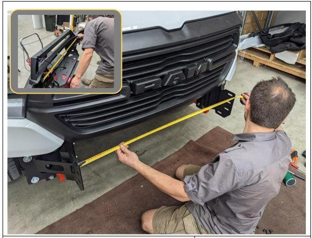
50. Measure Distance between outside edges uprights on bar using tape measure. Write distance below for reference if required.
