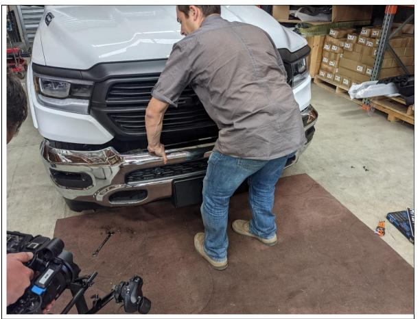
7. Remove front bumper by lifting forward off the car.
