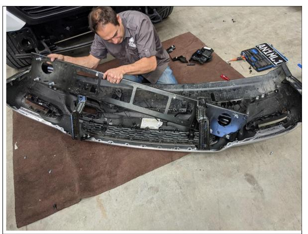
21. Remove the center beam from the bumper. This will give better access to the parking sensors for removal.
