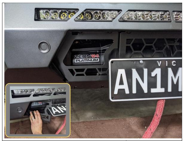
74. Fit Mesh Infill Panels. Use 2x M8x16 Button head bolt, M8 flat washer and M8 flange nut for top mount.
