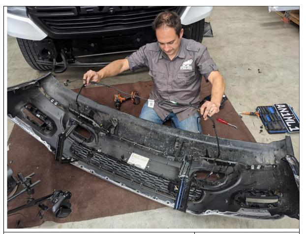
25. Remove the loom from the lower bumper, by prying off all clips securing the loom to the bumper with a trim tool.
