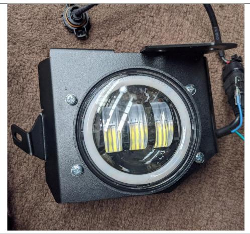
32. If fitting optional halo fog lights, Fit Halo fog lights to the fog light brackets using the M4 Hardware supplied.
