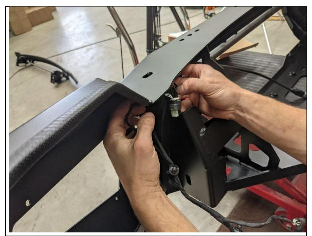
28. Pass wiring loom through bar uprights, starting from the left-hand side of the bar.
