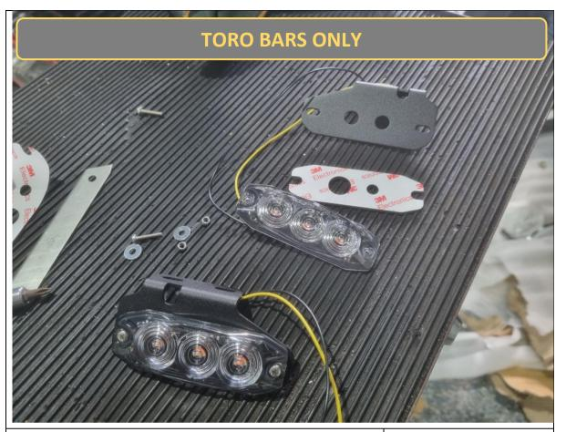
33. Fit the indicator repeater lamps to the indicator brackets, using M3 Phillips head Screws and the adhesive backing included with the lamp module.
