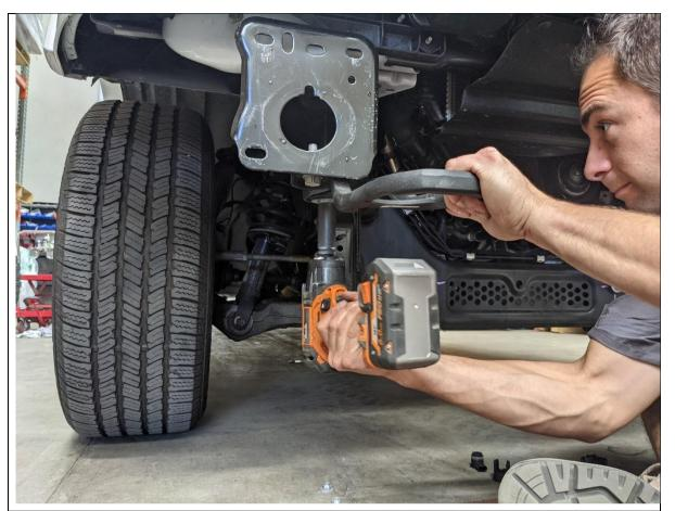
11. Remove the factory tow hooks, by removing the Factory Fine pitch bolts securing it to the chassis.
