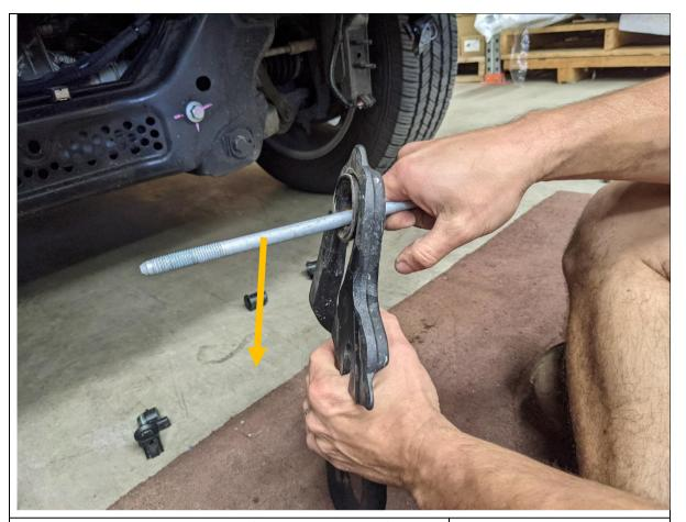
12. Remove the rubber bushes from the back side of the factory tow points by pushing down through center of bush with long factory bolt as shown in image above.
