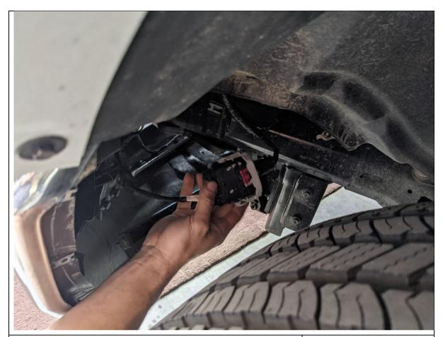
6. Disconnect the fog light and parking sensor loom, located underneath the LH headlight.
