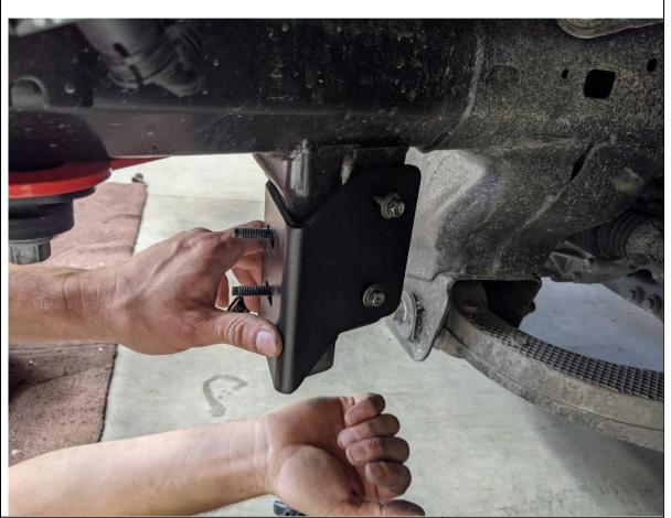
19. Fit the Bash Plate Mount Bracket to the chassis, Using Factory flange nuts and bolts removed from the inner guard liner and active air dam.
